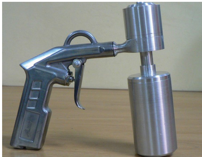
■ A prototype device for fine dispersion spraying with simultaneous heating or cooling of the sprayed substances (developed under a state contract with the Ministry of Defence of the Russian Federation)
